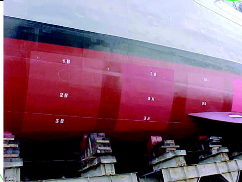
Below: Co-Biocide test patches applied on the side of USS RENTZ.
